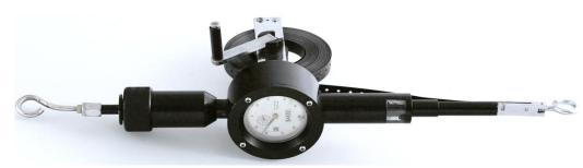
second reference anchor. Now the slack of tape is reduced to minimum possible by fixing the punched hole on the pin provided on the instrument. The fine and final setting of tape is done by tightening the tensioning knurlad nut till the index marks provided on the instrument are aligned perfectly. This gives final measurement between two points always at a fixed tension on tape.
