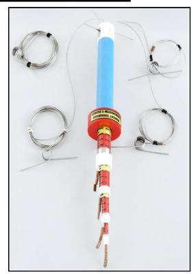
After installation of all anchors the anchor pipe assembly with spring will be inserted into hole leaving all the scale hanging one in each. When the bed /roof separation is taking place the reading will change in respective scales.
