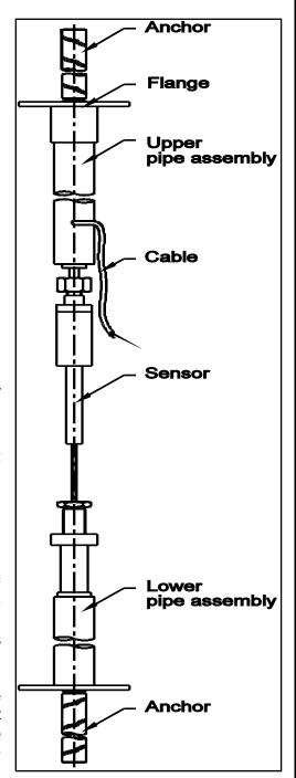
Top flange assembly is provided with height adjustment extension pipes to suit cavity height. Basic assembly height is 2 meters.
