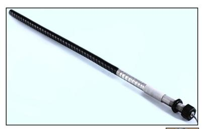
installed in the normal manner, making sure that the strain gage remains located within the loaded part of the rock bolt. Strain in the rock bolt is converted to equivalent loads using calibration coefficients supplied with the equipment.
