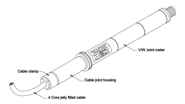
**CAUTION:** Make sure that the threads of the joint meters are not damaged in transport or storage. They should match with the threads in the joint meter and the socket assembly.
