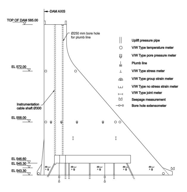
NOTE: IS: 7436 (Part II) states – "In the case of large dams built in V-shape canyon, joint meters should be provided in at least three blocks, namely, deepest central block and a block each in the abutment portion representing blocks built on steeply sloping abutments. In plan of a given elevation the joint meters in each of these blocks should be installed on the center of the longitudinal joints and at the center of the transverse dimensions of the monoliths in the block, spaced about 15 m
