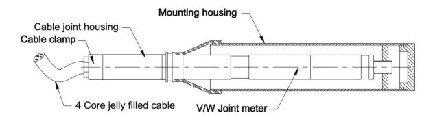
**a.)** Remove the cable joint housing from the cable end of the sensor. This gives access to a four cable. Two of the wires red and black colors are connected to the coil of the vibrating wire sensor. The other two wires green and yellow connect to a thermistor used for temperature measurement.
