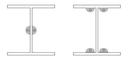
Sheet Piles Install gauge on both sides of the pile, awqzy from the clutches.
